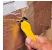
Above: Shrink Wrap Cutting Tool. A safer alternative.
