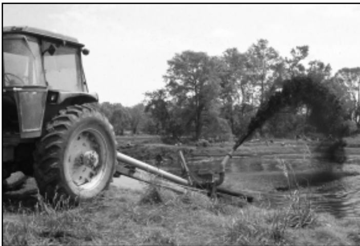
Figure 4. Agitator pumps are very efficient for suspending, mixing, and removing sludge from a lagoon to a tanker or irrigation pump. Special care should be taken to prevent erosion of the lagoon walls when operating the recirculation nozzle.
