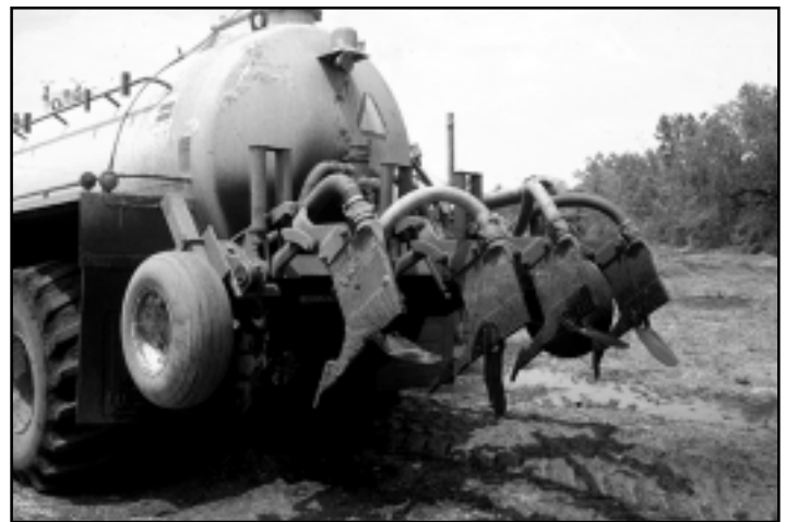
Figure 6. Injecting sludge directly into the soil reduces odors but increases the cost and time of application.
