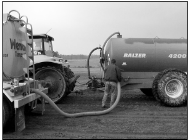
Figure 5. Tankers reduce the cost and time of applying sludge to fields that may be miles from the lagoon.
