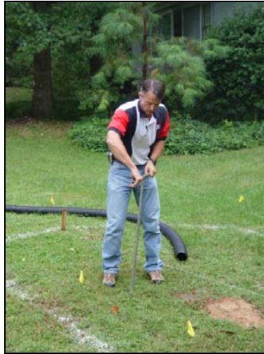
Figure 5.2 A rain garden's perimeter is laid out and a soil test is taken.
