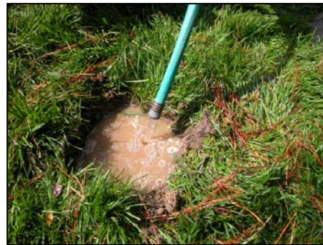
Figure 3.9 Simplified soil infiltration test
