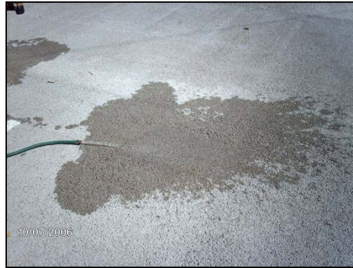
Figure 10.1 Illustration of permeable pavement function – garden hose dispensing onto permeable concrete
