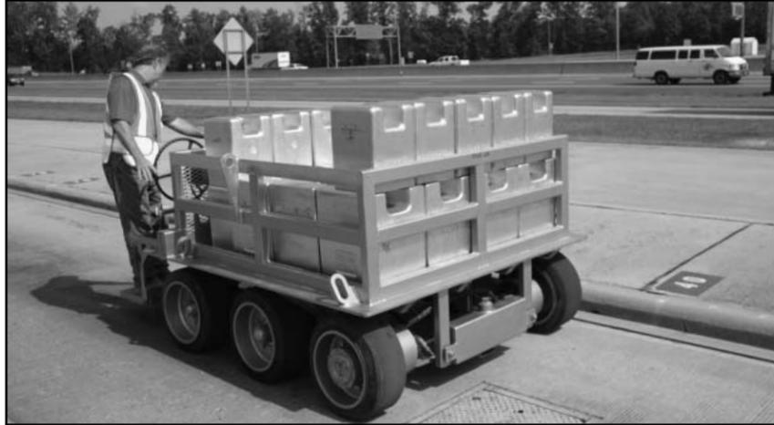
An NCDA & CS Standards Division inspector positions the 5,500-pound steel test cart on the truck scales to check the weigh-station equipment for accuracy.
