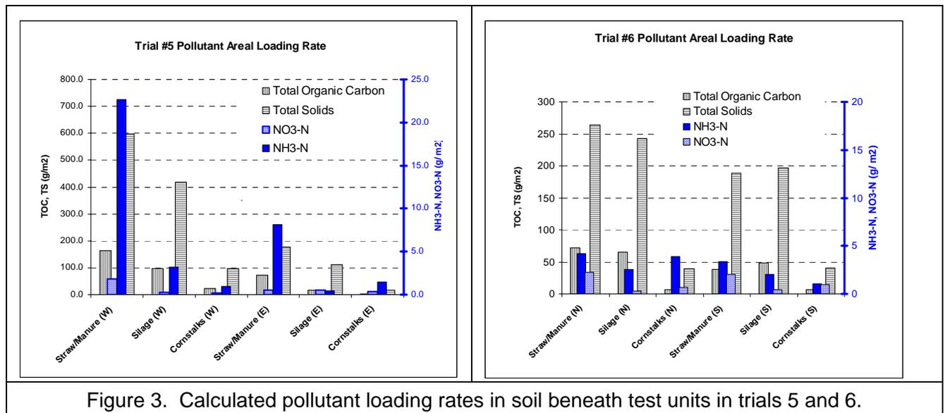
Figure 3. Calculated pollutant loading rates in soil beneath test units in trials 5 and 6.
