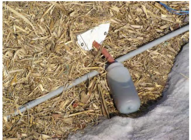
Figure 1. Gravity flow leachate collection troughs (left) and polyethylene leachate bottles (right) used to capture leachate samples during trials 5 and 6.
