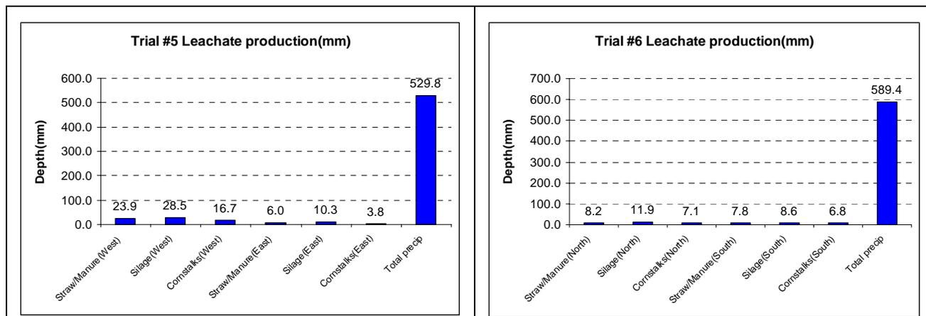
Figure 2. Total depth of leachate captured beneath test units in seasonal trials 5 and 6 compared with concurrent precipitation.
