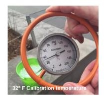
5. If the dial does not read 32°F, using the flathead screwdriver, turn the small (1/4") hex screw head on the back of the dial case of the thermometer until the pointer is at 32°F. Turn the screw counter-clockwise to increase temperature or clockwise to decrease temperature.
