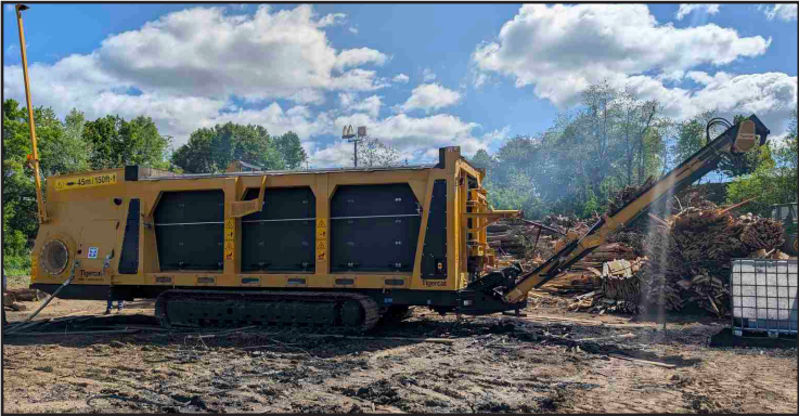
A carbonizer is used to heat organic biomass material and convert it into biochar.
