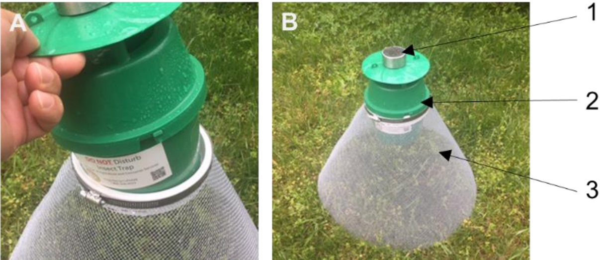
Figure 4.3, a. Details of the sweet potato weevil trap to use in the MAT. b. The base of the trap is a funnel made with galvanized mesh (3). This allows weevils to walk to the bucket trap fitted within a PVC ring that holds the funnel (2). The bucket trap includes a solar cell (1) that charges an LED diode that produces a green light shown to attract more weevils. The diode is activated late in the evening when weevils are active and deactivated when there is sunlight.
