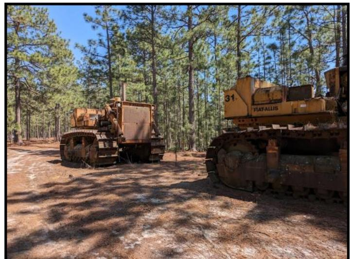
Heavy machinery located on sandy soil that is dry enough to support the equipment weight without rutting.
