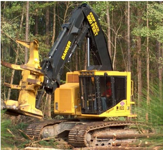
*Left: A track-mounted tree harvesting machine (called a tracked feller-buncher).*
