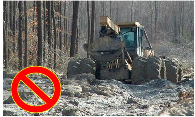
Skidders should only run on the shovel trail (left), and not directly on the bare ground of the swamp (right).
