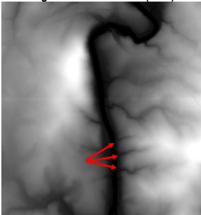
DEM maps look similar to LIDAR and can be made from LIDAR point clouds. The DEM is a digital representation of ground topography, excluding vegetation and other surface features. The DEM is stored as an image (raster) and is continuous data rather than individual points like LIDAR.
