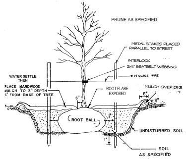
LOOSEN AND BLEND THE SOIL IN THE ENTIRE PLANTING AREA AS DIAGRAMED. THE PLANTING PIT SHALL BE 2 TIMES THE BALL DIA.
