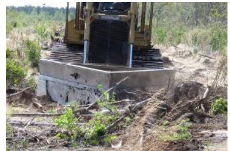
Bulldozer with V-blade pushing debris aside for bedding.
