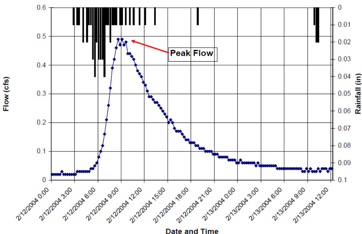
**Figure 3.6 Hydrograph with peak flow rate emphasized.**
